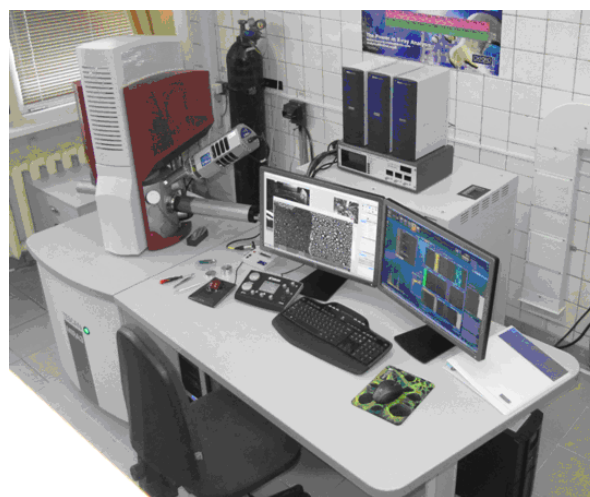
Fig. 1 Scanning electron microscope of high resolution "Mira-3" of "Tescan" company (Czech Republic)
