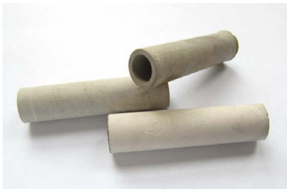
Fig. 5 The samples of permeable materials based on a granular mechanically activated alumina powder
