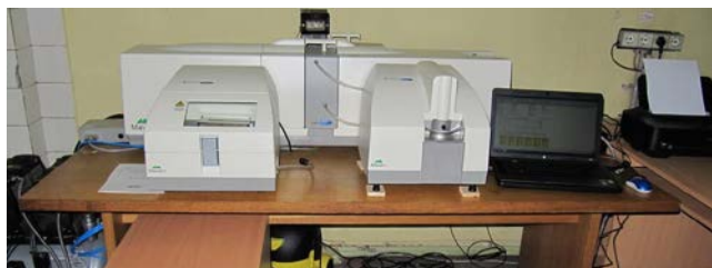
Fig. 6 Laser Diffraction Particle Size Distribution Analyzer Malvern Mastersizer 2000 with an automatic dispersion and delivery module of the HydroS sample for determining the fineness of purification
