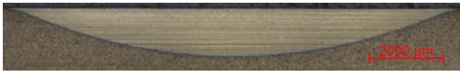
Fig. 2 The macrostructure of the surface hardened area in a perpendicular direction - field deflection.
