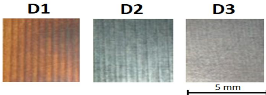
Fig. 1. Optical microscope image of \text{TiO}_2/\text{Ti} structure after irradiation by the laser doses D1 , D2 , and D3 at laser intensity 52.8 \text{ MW/cm}^2 .
