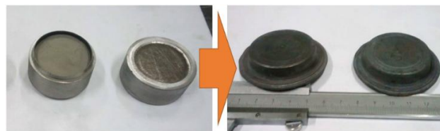
Fig. 1. Steel container with Inconel 625 powder before and after processing by the DPF scheme.
